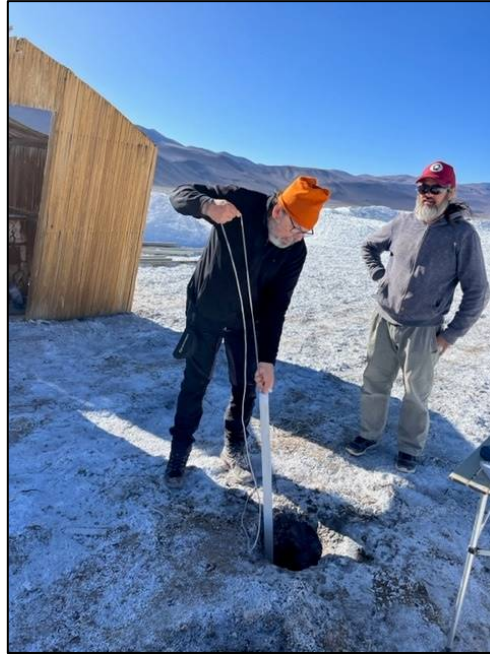
Photo 12-1: Obtaining sample SAL-003 using a bailer
