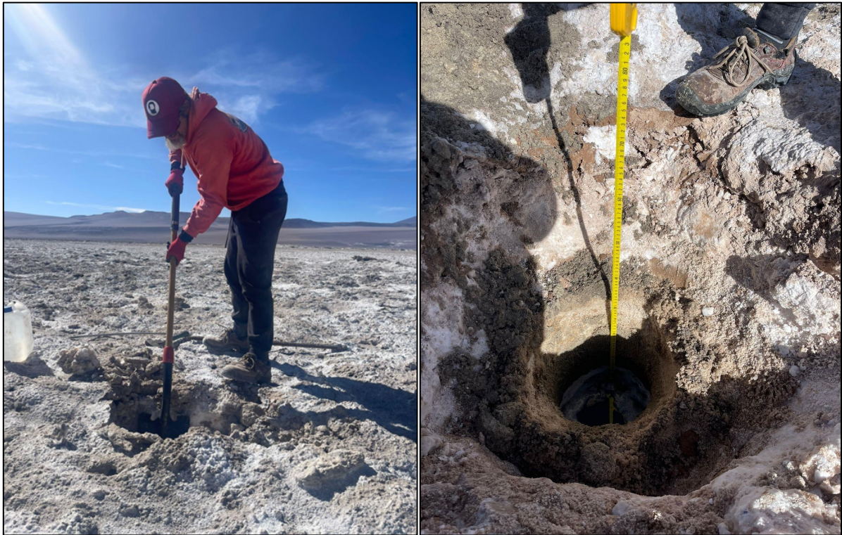
Photo 9-1: Left: Pit Excavation, Right: Water Level Measurement
