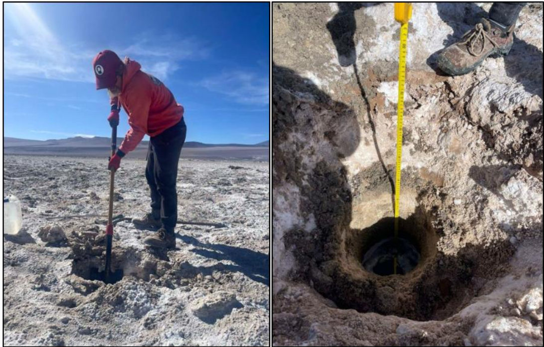
Photo 9-1: Left: Pit Excavation, Right: Water Level Measurement
