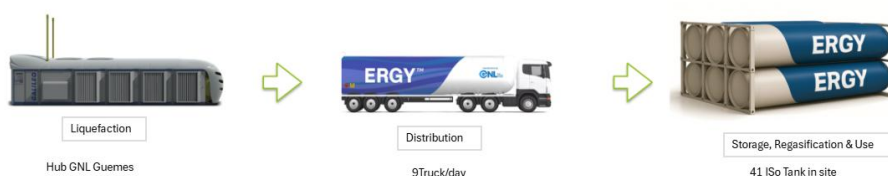
Figure 18-6: Schematic LNG transport and storage.
