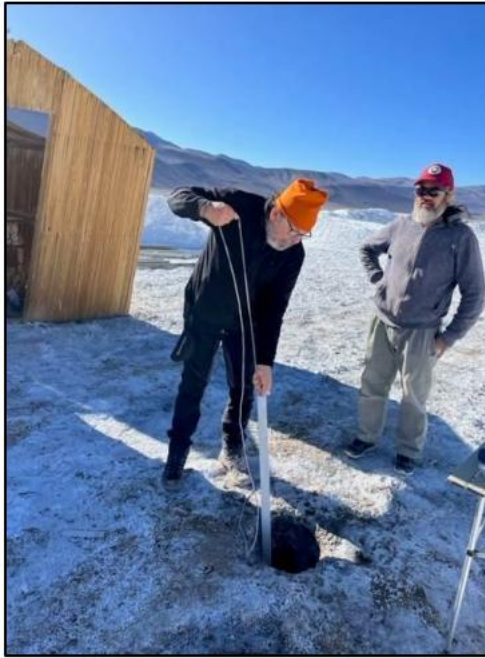
Photo 12-1: Obtaining sample SAL-003 using a bailer
