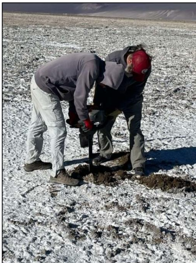
Photo 12-2: Using a Power Auger to Drill Down to Groundwater Level
